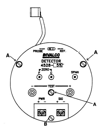
The Model 4528 Detector mounts in the explosion proof conduit on the capacitance probe. It converts water changes in the oil flowing through the probe to an output voltage that varies with the water.
