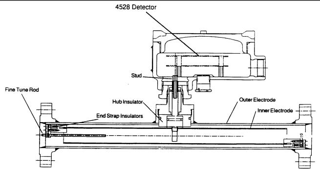
The probe is constructed of two concentric tubes. Wetted and internal surfaces are coated with a fused epoxy powder. The inner tube is insulated from the outer tube by Teflon spacers and is electrically connected to a terminal within the sensor housing. The internal element spacers can be fitted with trimmer rods should it be necessary to adjust the base capacitance.
