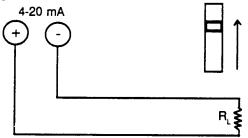
Loop switch is up in internal position on Model 4728 with terminal strip across bottom.
