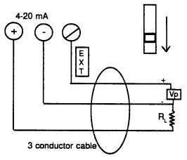
Loop switch is down in external position on Model 4728 with terminal strip across bottom. Loop switch is up in external position on CSA Approved 4728.\*
